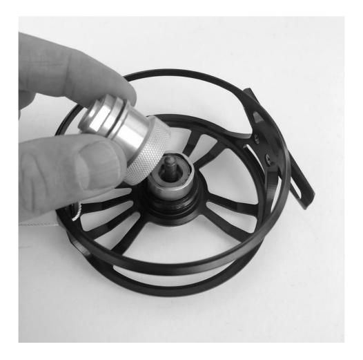
When you lift the brake housning you will now see the one-way bearing, BUT depending on the amount of grease inside the housning it can ither sit inside the brake housning (the part the hand is holding in the image), or inside the drag spindel in the bottom of the reel frame (the part in the centre of the reel frame).
